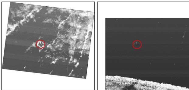
Figure 8: variation of the contrast with the Automatic Gain Control. Flight altitude: 30 m
