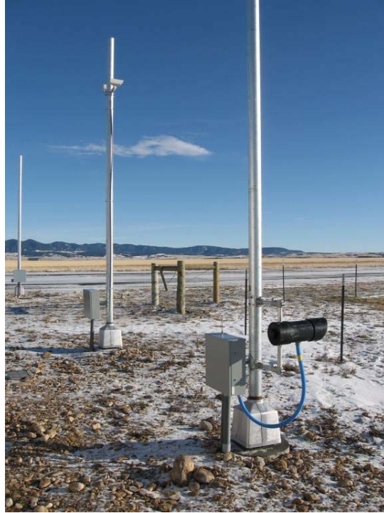
Figure 3.4: Some of the sensors of the animal detection systems (Photo: Marcel Huijser, WTI/MSU).
