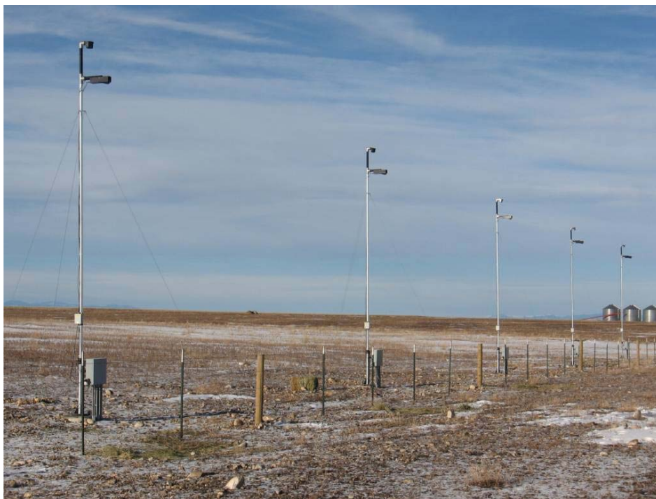
Figure 3.5: The infrared cameras that monitor animal movements in the enclosure (Photo: Marcel Huijser, WTI/MSU).
