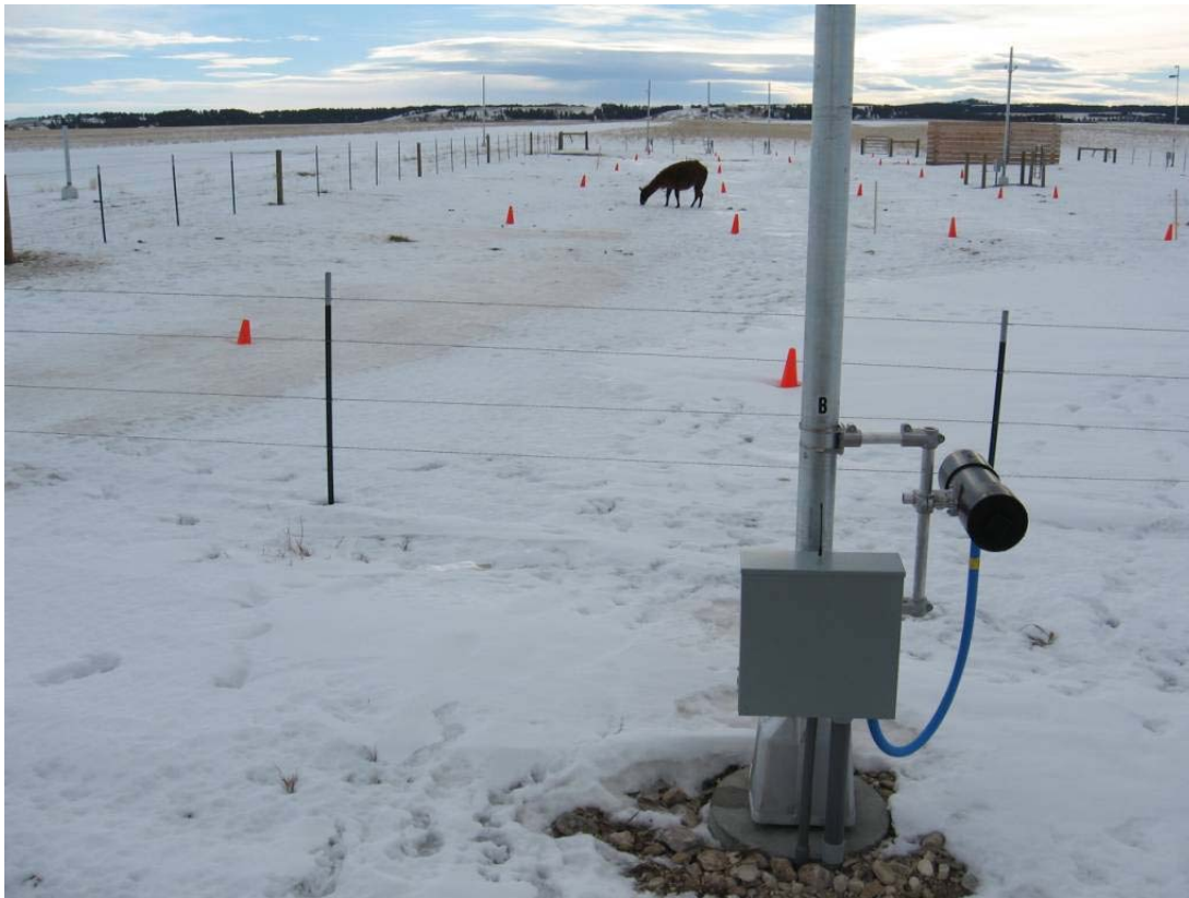
Figure 3.6: The detection zones and detection lines were marked with cones to be able to record the position of the animals (Photo: Marcel Huijser, WTI/MSU).
