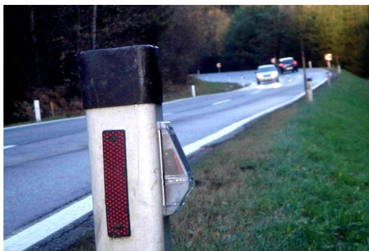
Figure 17. Virtual fence sensor attached to a roadside post (Reid, 2012).
